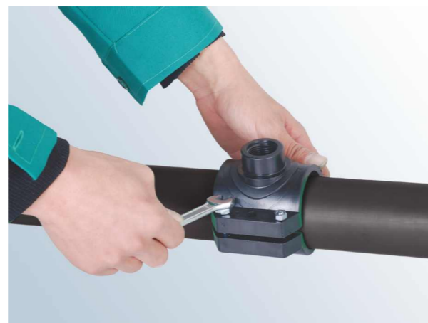
6. Assemble the saddle according to the marked lines, to keep the hole in the same axis with the saddle's screw hole.
