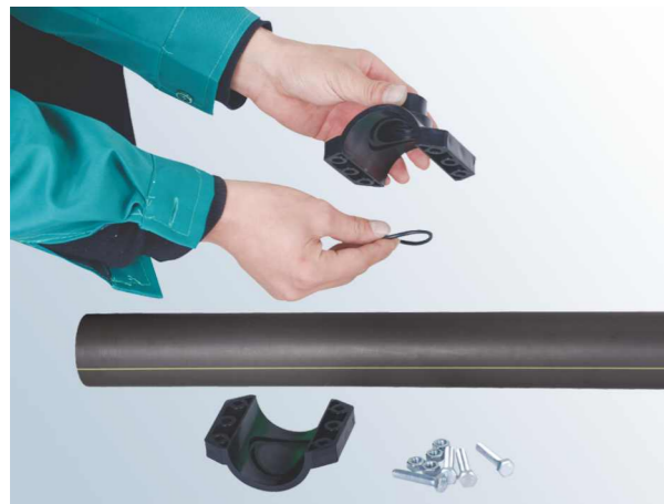
1. Select the hole point and make sure that the external surface of the pipe is free from any impurity, put the gasket into the indentation of the saddle seat.
