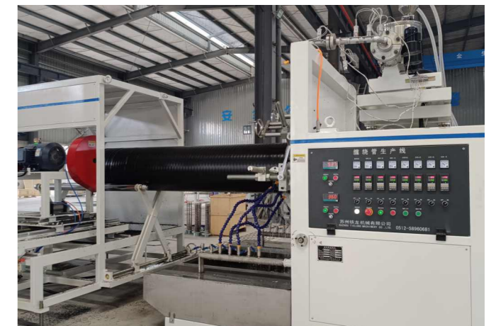
Hollow Wall Winding Pipe Production Workshop
