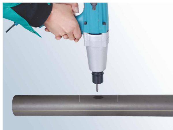
5. Drill the hole in the pipe wall being carefull not to damage the other side of the pipe and remove the scraps.
