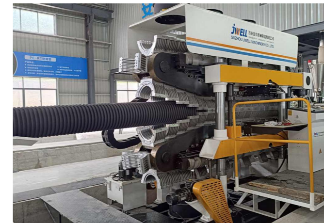
Double Wall Bellows Production Workshop
